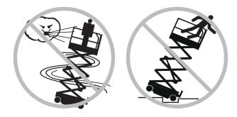
Do not drive the machine on or near uneven terrain, unstable surfaces or other hazardous conditions with the platform raised. Use extreme care and slow speeds while driving the machine in a stowed position across uneven terrain, debris, unstable or slippery surfaces and near holes and drop-offs.
